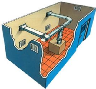
Typical Flue Dilution
